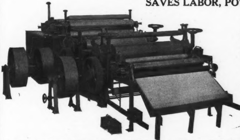
Illustration shows Rogers Double Wet Machine which has a capacity of 30 dry tons in 24 hours.
